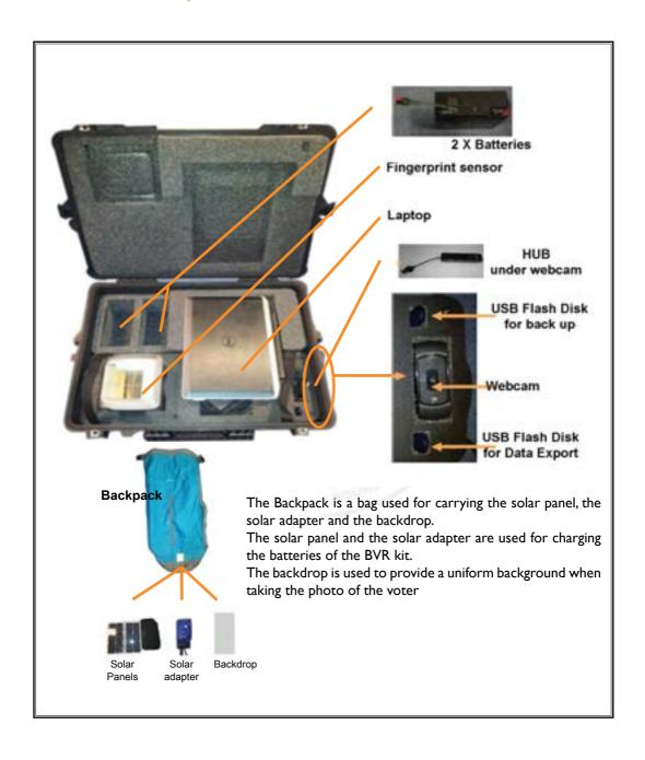
The registration kit is composed of a laptop, fingerprint scanner, webcam, hub, two rechargeable batteries and two flash disks. The kit stored in a waterproof and shockproof storage case. The fingerprint scanner, the webcam, the hub and the two flash disks are stored in a separate movable container (plate) within the case. This container also contains power connections to the batteries and the laptop.
