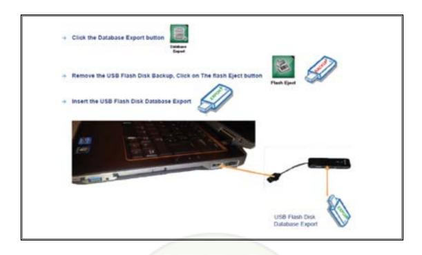
Step 5: Insert the flash disk B into the USB hub to export the data.
